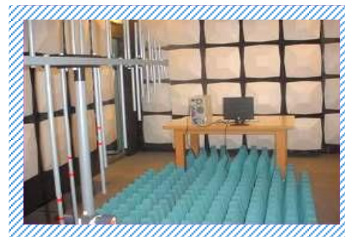
RS Test Setup(743 Chamber)
